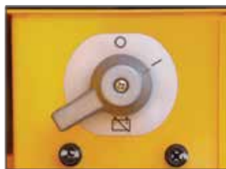
BATTERY DISCONNECT SWITCH
